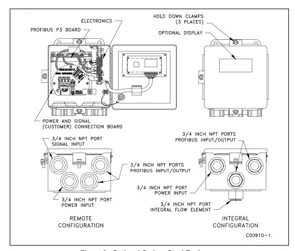
Figure 8. Optional Carbon Steel Enclosure
