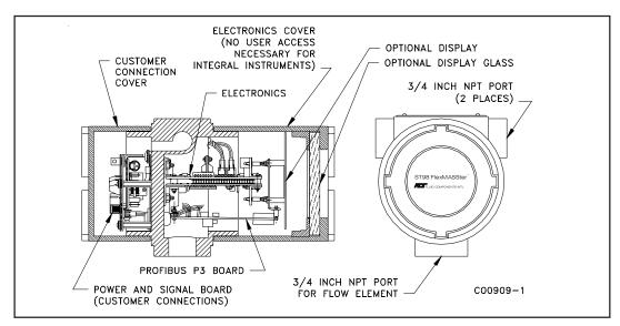
Figure 5. Circuit Board Placement
