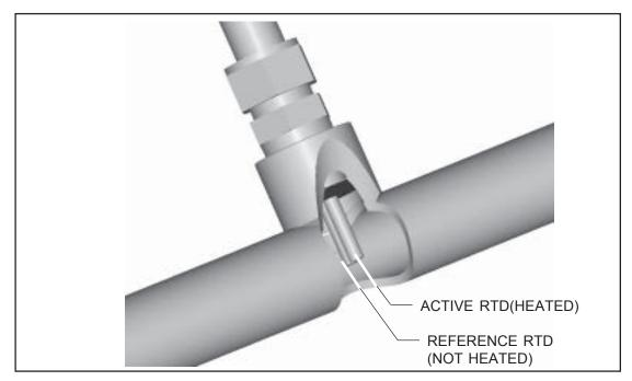
Figure 2. Cut-Away View Of The In-Line Flow Element Tube
