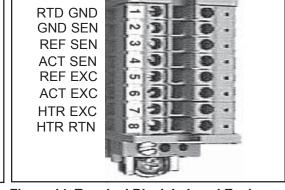
Figure 13. TS2 Connector Plug
