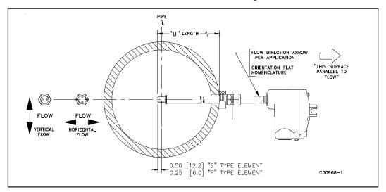
Figure 3. Model ST98 Insertion Flow Element (Remote) Showing Orientation
