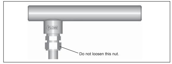
Figure 4. Model ST98L In-Line Butt Weld Mount
