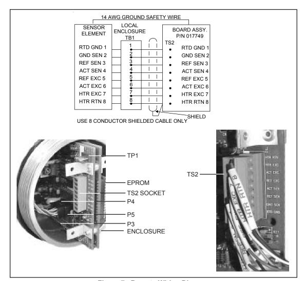
Figure 7. Remote Wiring Diagram
