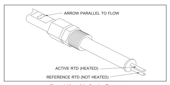
Figure 1. View of the Sensing Element
