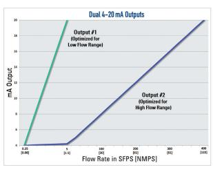
Figure 3: Dual Calibration Performance
