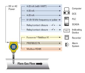
Figure 5: Readouts & Digital Communication
