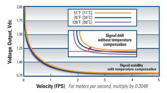
Figure 2. Temperature Compensated Flow Curves
