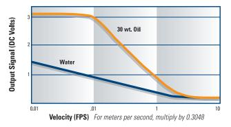
Figure 3. Typical Liquid Flow Curves
