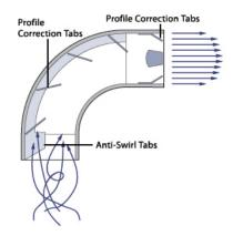
Figure 2. Tube and Elbow Tab-Type Conditioner
