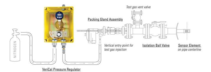
Figure 5: ST110 Flow Meter with VeriCal In-Situ Calibration System
