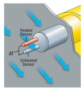
Figure 3: Thermal mass flow sensor element
