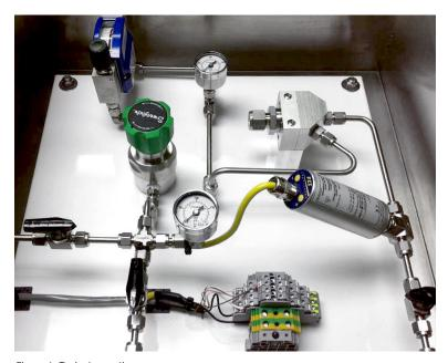
Figure 1: Typical sampling system
