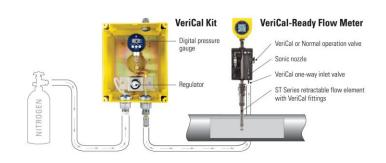
San Marcos, CA—The breakthrough ST100 Series Thermal Mass Flow Meter from Fluid Components International (FCI) is now available with FCI's VeriCal In-Situ Calibration Verification System, combining advanced measurement capability with the convenience of in-
