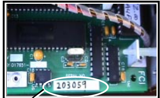
Electronics Serial Number (Located on the circuit board with the larger I.C. chips. It is also on the transmitter's (FT) enclosure tag.)
