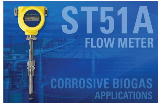
This meter's advanced electronics are housed in a durable NEMA 4X, IP67 dust/water ingress protected all-metal (aluminum or 316L stainless steel) enclosure with dual conduit ports in either NPT or M20 threading. The transmitter can be integrally mounted with the flow element (probe) or can be remote mounted for installation flexibility. The instrument comes standard with dual 4-20 mA, NAMUR NE43 compliant outputs and a 500 Hz pulse output.
