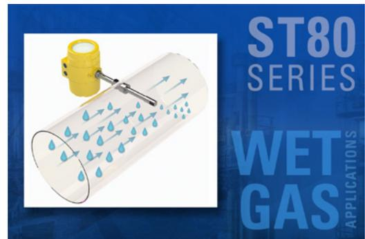
Eliminating the moisture from the gas stream is always the preferred, best practice when possible. Common moisture removal methods include installing gas dryers or knockout drums or knockout pots upstream from the flow meter. Many times, however, these techniques are either infeasible due to crowded equipment areas or awkward pipe configurations.
