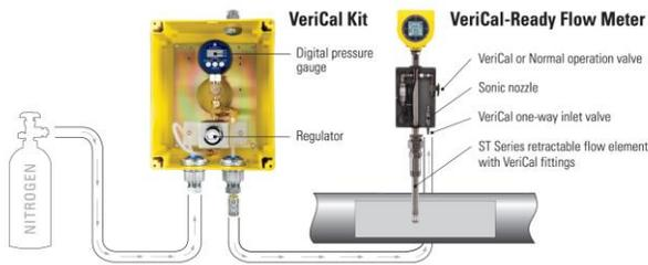
San Marcos, CA — Oil/gas engineers responsible for performing routine flow meter calibration verifications who want to eliminate the hassle and cost of shutting down the line, pulling the meter, installing a spare and paying a lab fee will find the [VeriCal™ In-Situ Calibration Verification System](#) with the [ST100 Series Thermal Mass Flow Meter](#) from [Fluid Components International \(FCI\)](#) eliminates all the problems.
