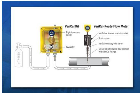
San Marcos, CA — With the [VeriCal In-Situ Calibration Verification System](#) for the [ST00 Series Flare Gas Flow Meter](#) from [Fluid Components International \(FCI\)](#), offshore oil/gas process engineers and operators can now eliminate the time-consuming and costly task of traditional flow meter calibrations, which require shutting down the line, pulling the meter, installing a spare and
