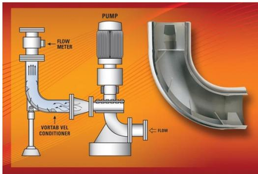
**San Marcos, CA** — Process and plant engineers who can't find room for the recommended straight pipe run required by liquid flow meters in their municipal water treatment plant retrofit projects will find the [Vortab Elbow Flow Conditioner](#) from [The Vortab Company](#) eliminates the problem by removing swirl and asymmetric velocity profiles
