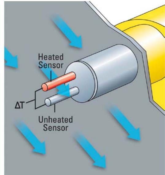
Figure 3: Thermal dispersion constant power principle of operation
