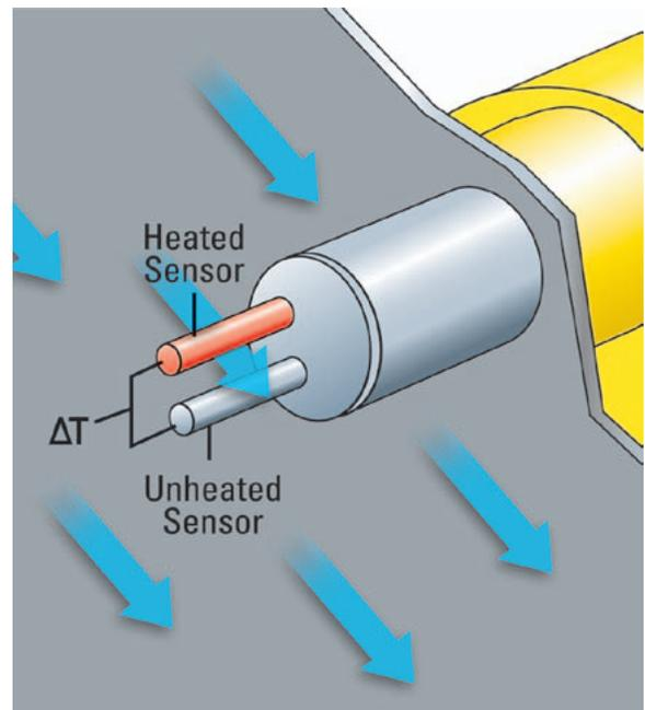
Figure 4. Thermal Dispersion Mass Flow Measurement
