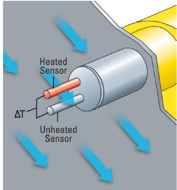
Figure 3. Thermal Dispersion Mass Flow Measurement
