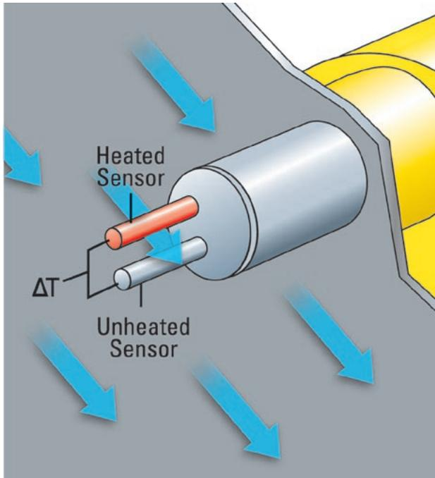
Figure 2. Thermal Mass Flow Sensing Theory of Operation
