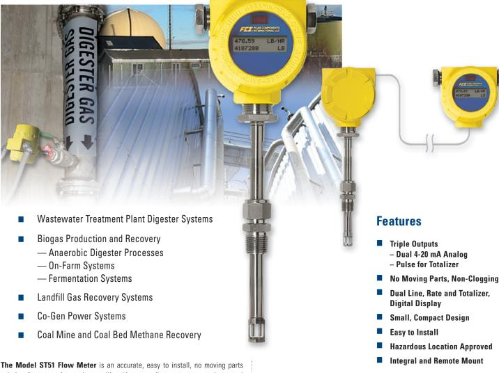
**The Model ST51 Flow Meter** is an accurate, easy to install, no moving parts solution for measuring and controlling biogases, digester gases, methane and natural gas flow. Model ST51 utilizes FCI proven thermal dispersion technology to provide direct mass flow measurement resulting in higher performance at a lower cost than orifice plates, DP, Vortex shedding and other thermal devices.
