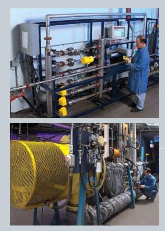
More than 16 precision flow stands to match fluids, process conditions, flow rates and line sizes specified in your application.
