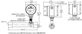
**Female NPT Configuration** DIM C Flow CL to Bottom DIM A Pipe Size DIM D VMR Length DIM B Configuration Top to Flow CL ST75V-XXXCE 1/4″ 5.50 [140] 0.38 [9,5] 5.00 [127] ST75V-XXXEE 1/2" 5.69 [144,5] 0.57 [14] 7.50 [190,5] ST75V-XXXFE 6.45 [164] 3/4" 9.00 [229] 0.69 [17,5] ST75V-XXXGE 1″ 6.44 [163,5] 0.88 [22] 9.00 [229] 1 1/2" ST75V-XXXHE 6.42 [163] 1.25 [32] 13.50 [343] ST75V-XXXJE 2″ 6.43 [163] 1.50 [38] 18.00 [457]
