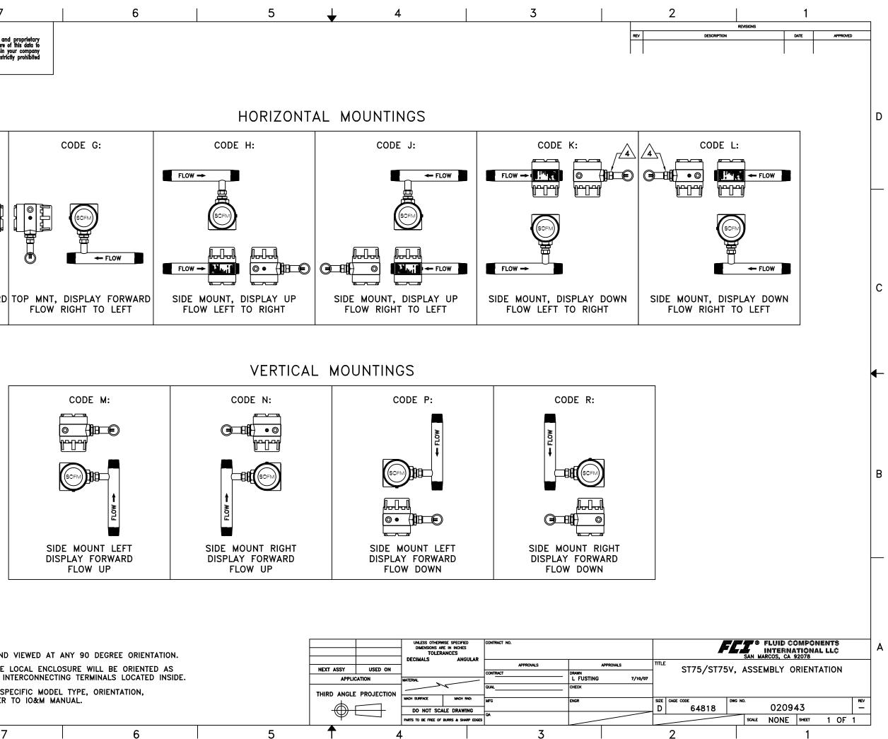
4 FLOW ARROW ON TOP AS SHOWN Α 3. THE LCD DISPLAY CAN BE USER ROTATED AND VIEWED AT ANY 90 DEGREE ORIENTATION. 2. IN REMOTE ELECTRONIC CONFIGURATIONS, THE LOCAL ENCLOSURE WILL BE ORIENTED AS SHOWN WITH SOLID COVER ON BOTH SIDES. INTERCONNECTING TERMINALS LOCATED INSIDE. 1. THIS DRAWING IS GENERIC IN NATURE, FOR SPECIFIC MODEL TYPE, ORIENTATION, CUSTOMER PROCESS CONNECTION, ETC, REFER TO IO&M MANUAL. NOTES: UNLESS OTHERWISE SPECIFIED 7 8
