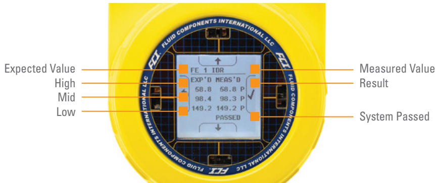
Figure 2: Front panel; all three check points show “P” (pass) and entire self-check “PASSED”
