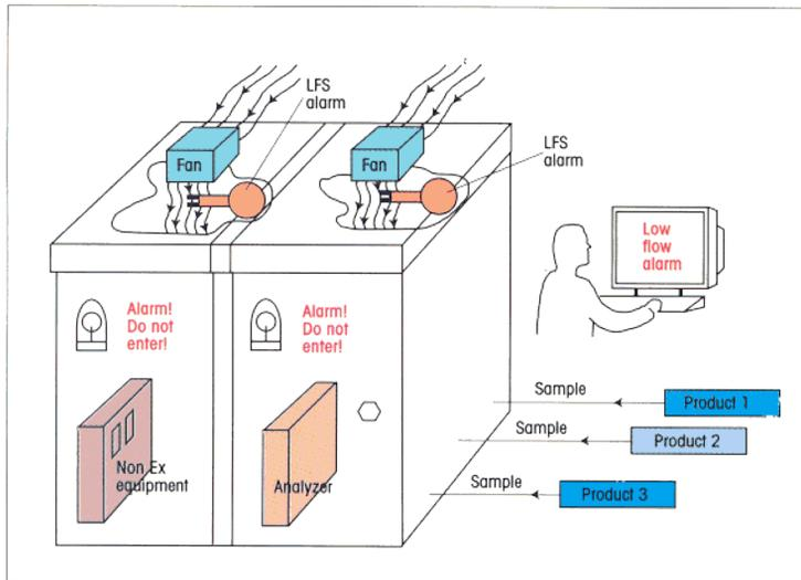
**FIG. 2:** If the air inlet flow drops below a preset value in an analyzer house, alarm lights at the entrance door are activated to warn people of an unsafe situation. A remote operator also receives the signal so equipment can be shut down.
