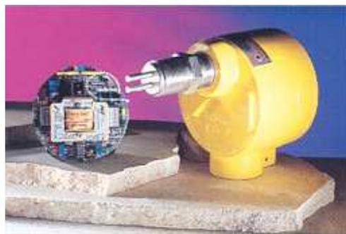
**FIG. 4:** The switch's control circuit is a fail-safe, dual-relay circuit board that is user friendly. Sensing elements are constructed of stainless steel, Hastelloy C276, Monel, or Titanium.
