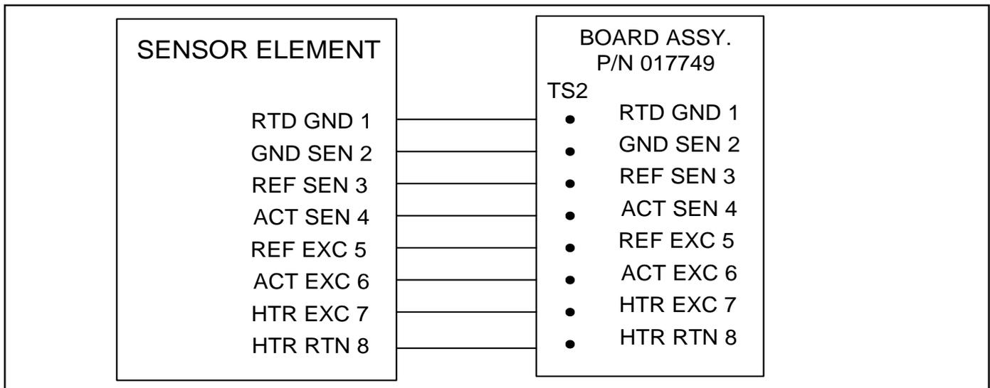
Figure A-8. Integral Option Wiring Diagram
