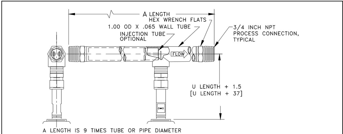
Figure A-7. In-Line NPT Process Connection
