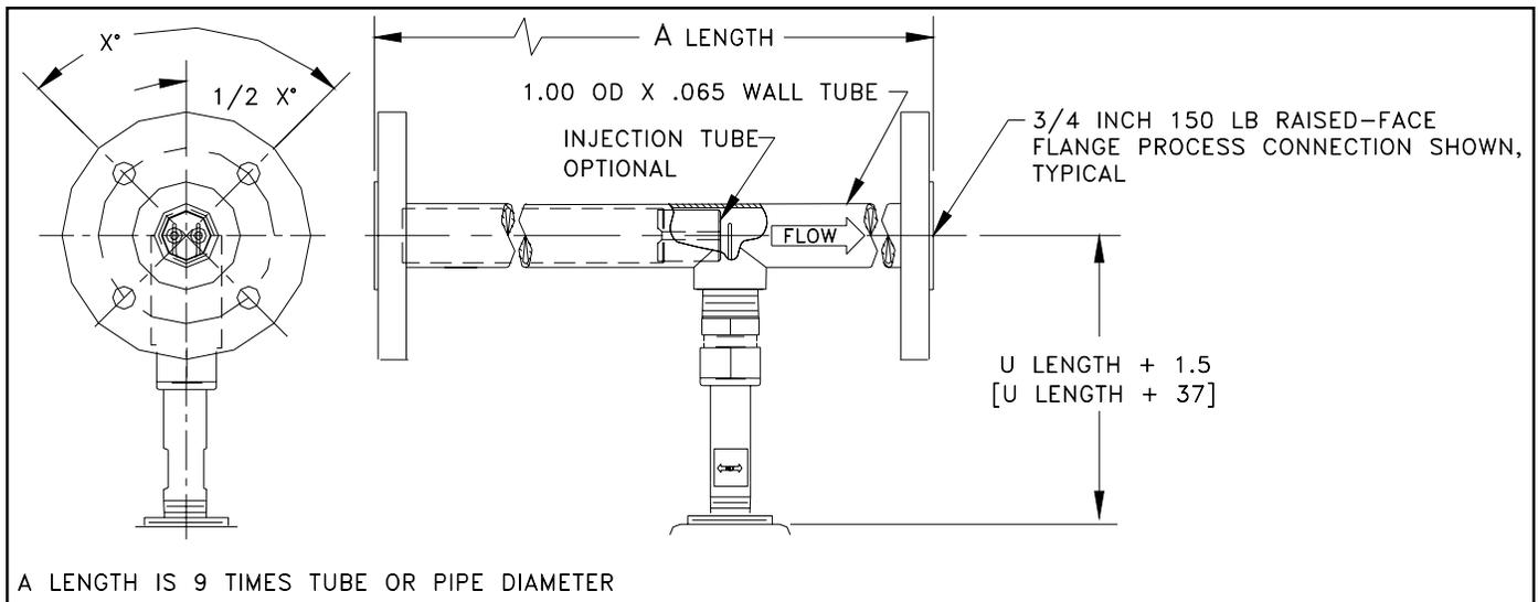
**Figure A-6. In-Line Flanged Process Connection**
