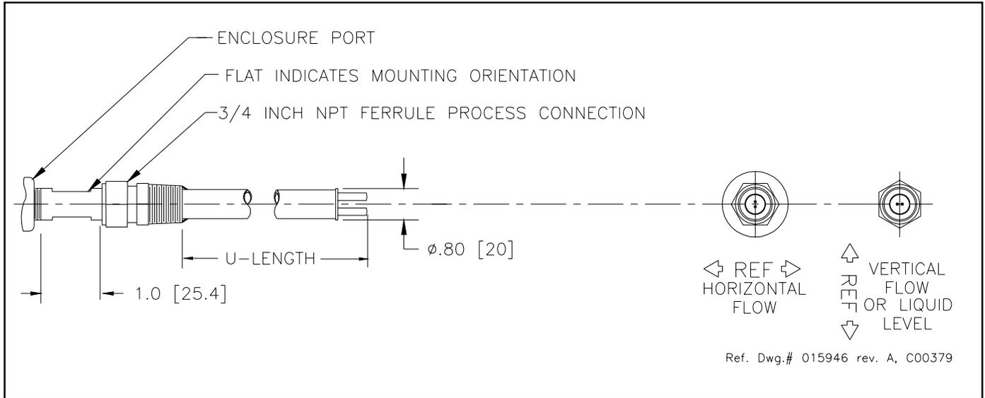
**Figure A-4. 3/4 Inch Ferrule NPT Process Connection**
