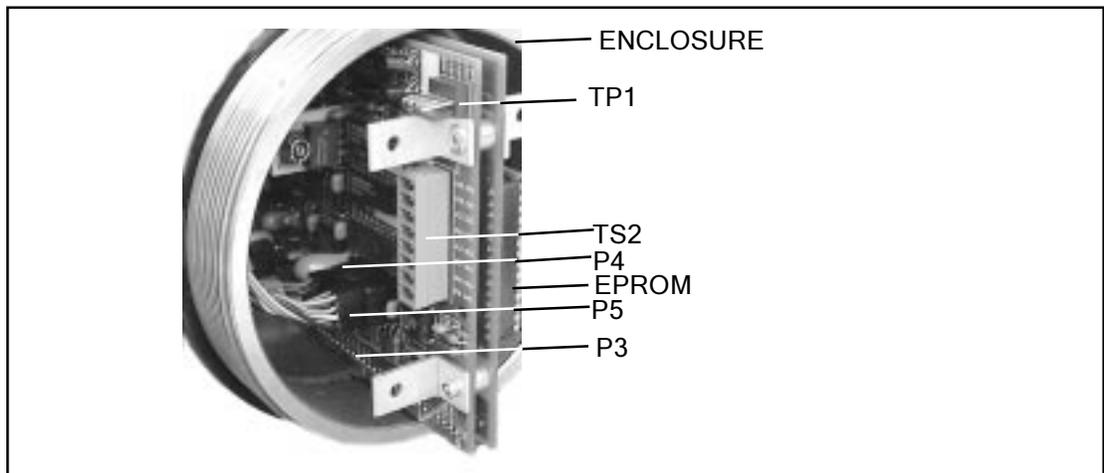
Figure 5-1. Component Identification
