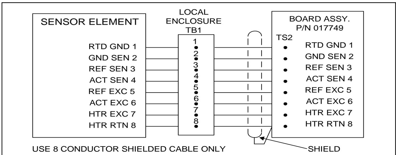
Figure A-9. Remote Wiring Diagram
