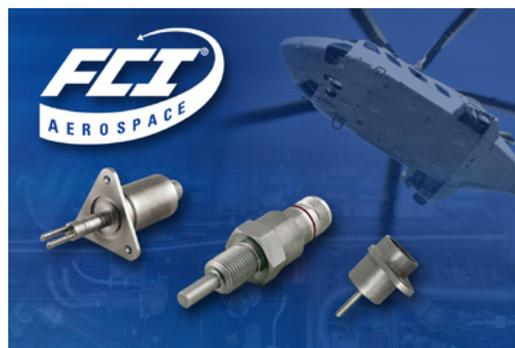
For example, FCI's AS-FS Series flow switches utilize no moving parts and ultra-reliable thermal dispersion flow measurement technology to detect a flow rate above or below a predetermined set-point at the sensing location. They are applied to signal low flow or high flow alarm conditions in air or liquid fluid flows throughout most airborne fluid systems.
