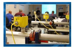
ST80 Series Flow Meter. FCI's WG sensor delivers accurate, repeatable gas flow measurement in the presence of moisture and condensation droplets. It can be applied for use in entrained moisture and rain-shielding applications.
