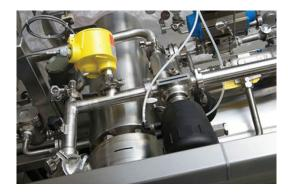
The sanitary FLT93C Thermal Flow Switch, with its stainless steel wetted materials and standard 20Ra finish, available in either mechanical polish or electro-polish finishing, supports
