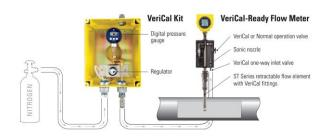
San Marcos, CA — Oil/gas engineers responsible for performing routine flow meter calibration verifications who want to eliminate the hassle and cost of shutting down the line, pulling the meter, installing a spare and paying a lab fee will find the VeriCal In-Situ Calibration Verification System with the ST100 Series Thermal Mass Flow Meter from Fluid Components International (FCI) eliminates all the problems.
