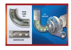
Upstream flow disturbers, such as elbows, expanders or reducers, and valves, often produce non-uniform, non-repeatable and swirling fluid flow entering the pump that can lead to pump cavitation and other issues causing premature wear. The result is extra maintenance, expensive repairs and/or premature replacement, which can take equipment offline. Vortab products provide effective <u>process conditioning</u> to protect pumps.
