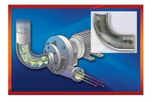
San Marcos, CA — Process engineers responsible for keeping the pumps running in plants crowded with equipment and awkward pipe layouts will find the <u>Vortab Elbow Flow</u> <u>Conditioner</u> is an effective, low-cost solution to eliminate the turbulent fluid flows that result in pump cavitation, which can lead to line shutdowns, expensive maintenance and shorter pump life.
