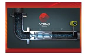
The <u>Vortab</u> flow conditioners overcome this challenge by delivering a uniform, swirl-free flow profile to the meter inlet in as little as a few pipe diameters for accurate, repeatable measurement. Upstream flow disturbers, such as pumps, elbows, expanders or reducers, and valves, often produce non-uniform, non-repeatable and swirling fluid flow entering the meter. These flow disturbers impact the flow sensor's ability to measure fluid flow accurately and consistently.
