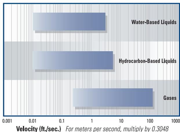
Figure 1. FCI Thermal Flow Switch Flow Ranges
